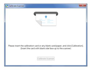
Note: Please make sure the blank side of the calibration card is facing up when placing it on the scanner. If the calibration card is lost, you may use a piece of blank business card or paper instead.
