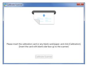
Note: Please make sure the blank side of the calibration card is facing up when placing it on the scanner. If the calibration card is lost, you may use a piece of blank business card or paper instead.
