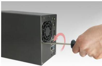
3. Position the bracket over the hole for the removed fan screw. Secure the bracket in place by replacing the fan screw.
