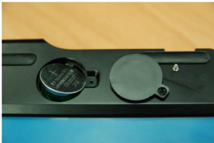
2. Put the new battery in, and then cover the battery cover and tighten the screw to finish.
