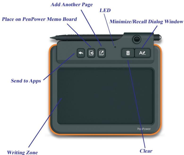
[Write2Go] uses the latest Boogie Board™ LCD eWriter technology, the real time display will shows your writing on the panel.
