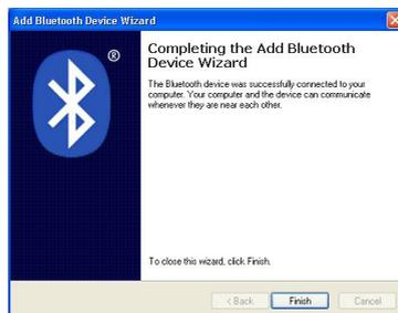
8. Then, the pen scanner will connect to your PC automatically. When pen scanner is paired with your PC successfully, the status light on pen scanner blinks slowly (blink every 3 seconds), and the pen scanner will connect with WorldPenScan BT automatically. You can begin to use WorldPenScan BT when the pen bluetooth status changed to **[Paired and connected]**.
