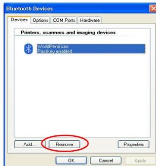
**Note 3:** For WorldPenScan BT, you can connect pen scanner with computer via USB cable and via Bluetooth at the same time. Follow the instructions to connect pen scanner with USB cable first, and enter the default passkey of pen scanner: 1234 in the Add Bluetooth Device Wizard directly, the pen scanner will connect to your computer automatically via Bluetooth. Now if you unplug the USB cable, you can continue to use pen scanner via Bluetooth.
