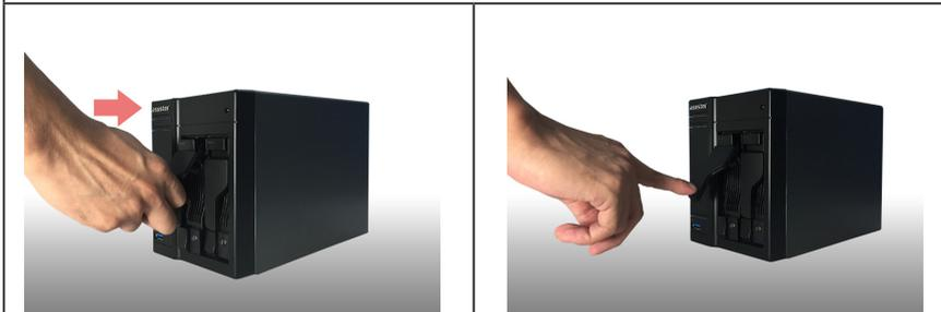
4. Once the latch is secure, you can lock it in place using the disk tray lock. Using a flathead screwdriver, turn the lock counterclockwise to lock the latch mechanism. Turning the lock clockwise will unlock it.
