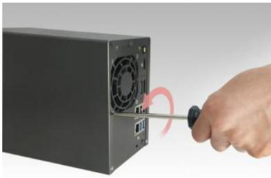
3. Position the bracket over the hole for the removed fan screw. Secure the bracket in place by replacing the fan screw.
