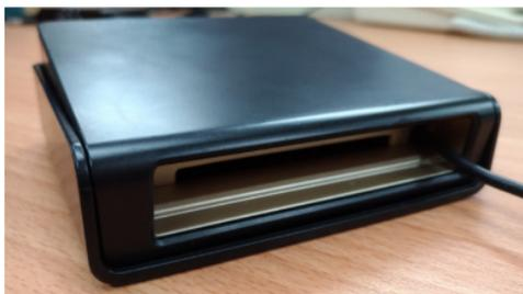
The cover of the card scanner must be completely lifted up first to expose the paper feed port, and then put the business card to the left to scan, as shown in the following figure.
