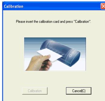
*Note: To calibrate the WorldCard Color and Office scanner, insert the blank side of the card face down. To calibrate the A4M Scanner, please insert the calibration card with blank side face up. The WorldCard Ultra plus color scanner doesn't need initial calibration, but if there is any color indifference, please insert the blank side of the card face up to calibrate it. In case the calibration card is lost, you can use any same size white card for calibration.*
